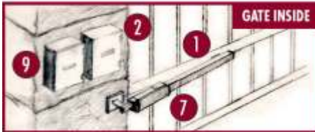
Gate Operator The swing gate operator (either gate mounted or in-ground) automates the gate
