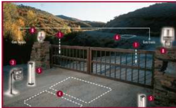
Photo-beams Photo-beams protect anything that "breaks" the beam ( vehicles, pedestrians, animals, children) which causes a reversal of the gate operators. Two sets of photo-beams are recommended for best coverage
